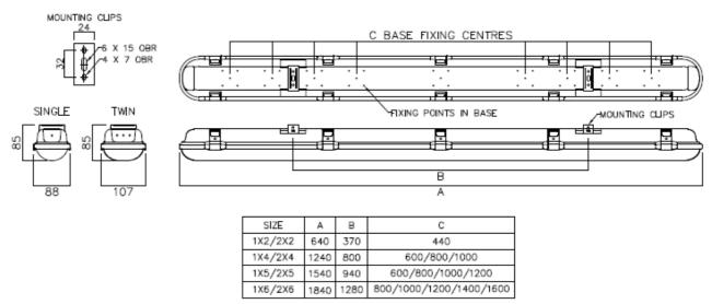
Surface fixing (using mounting clips\*): Mount the two stainless steel surface mount fixing clips provided (in accessory pack) to the ceiling at the specified fixing centres (see diagram). Offer the base up to the clips & push to snap fit.
